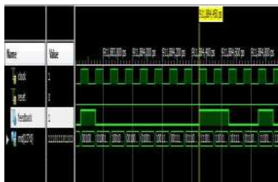
Fig.3. Simulated waveform for pseudo random number Generator using LFSR
